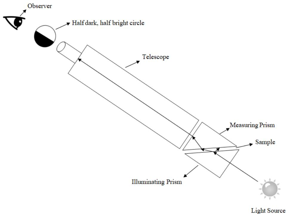
**Fig. 1: Schematic representation of Abbes refractometer**
