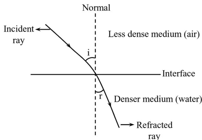
Fig. 1: Refraction of light ray.
