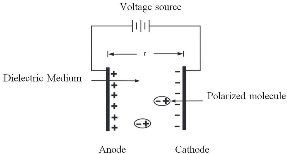
**Fig. 4: Parallel plate Condenser**
