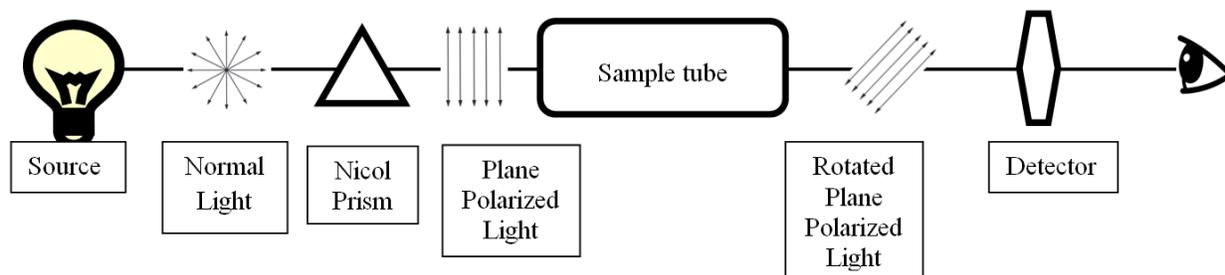
Fig. 3: Schematic presentation of Polarimeter
